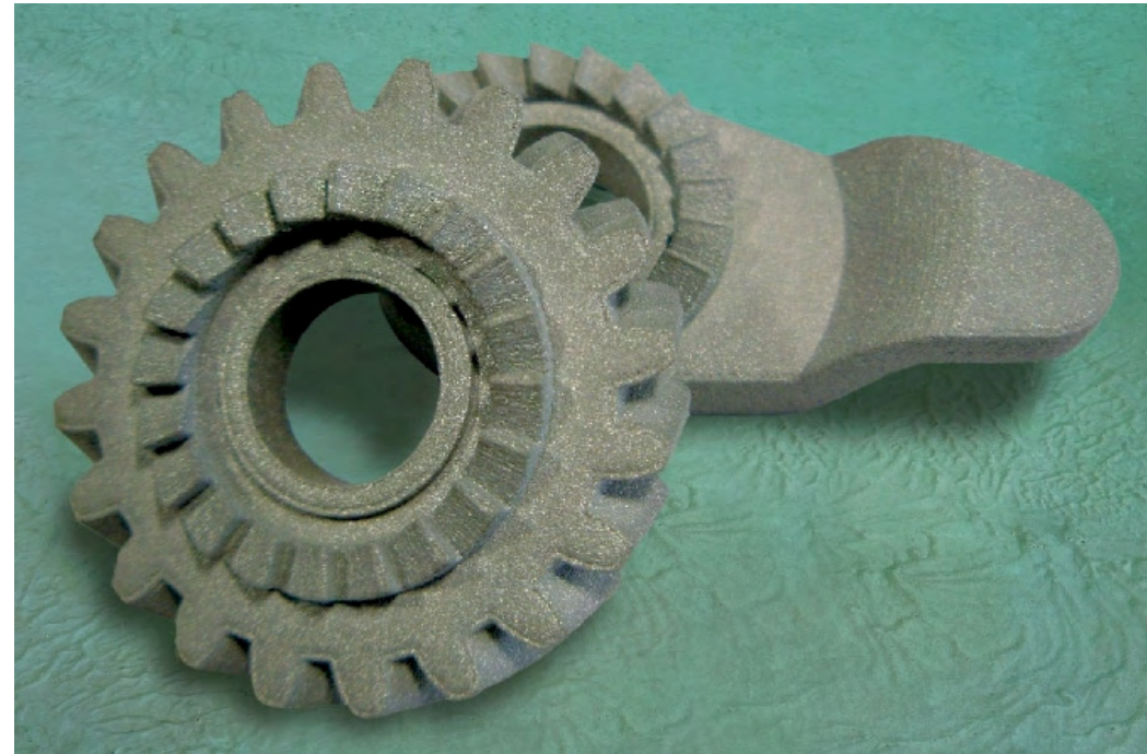
laser-sintered prototype of a door opener
