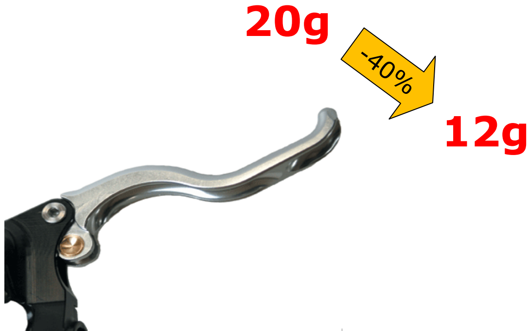
Conventionally manufactured brake lever in aluminium
