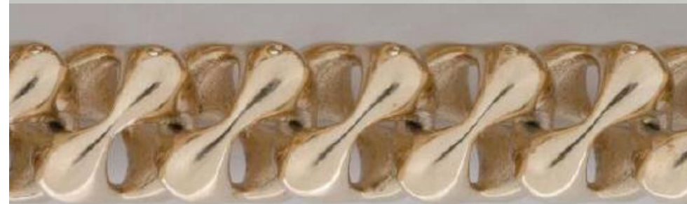
Charles chain. Above: silver, unpolished, 44 cm, 56 links. Below: gold plated silver, 40 cm, 52 links. Both built in one step on EOSINT M 250 Xtended. Design by Towe Norlén
