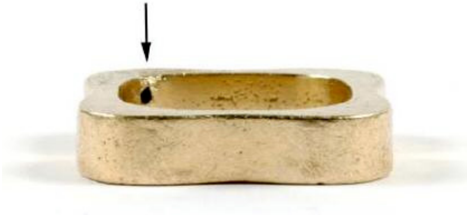
Flow, hollow ring, 18 ct yellow gold. Unsintered powder from the internal cavity was emptied out of the hole shown by the arrow, which could be soldered closed. The scratches are due to wearing the ring for two years. Design by Towe Norlén
