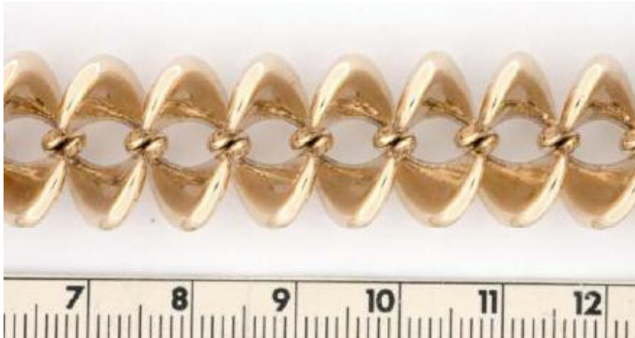
Fan chain in yellow 18 carat gold, 21 cm, 28 links. Built in one step on EOSINT M 250 Xtended. Design by Towe Norlén
